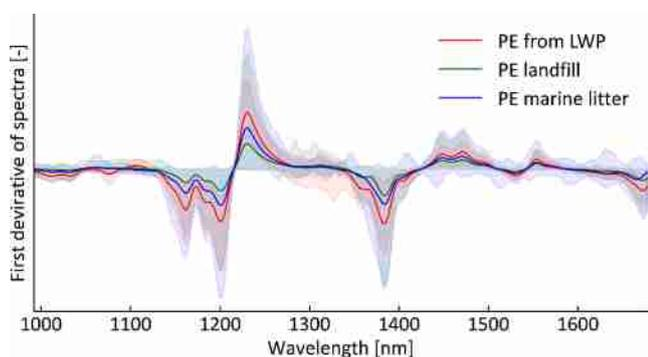
**Fig. 3.** Spectra of PE from different origins. Lines: mean spectrum of all 300 pixels; Colored range: spectra variation range.
