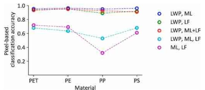
Fig. 4. Test score and classification accuracy of different materials according to degradation level with a component number of 15; ML: samples from marine litter; LF: landfill; Legend means classification between different classes, e.g. “LWP, ML + LF” means marine litter and landfill samples were grouped to one class and the classification was between LWP and the group of marine litter and landfill.
