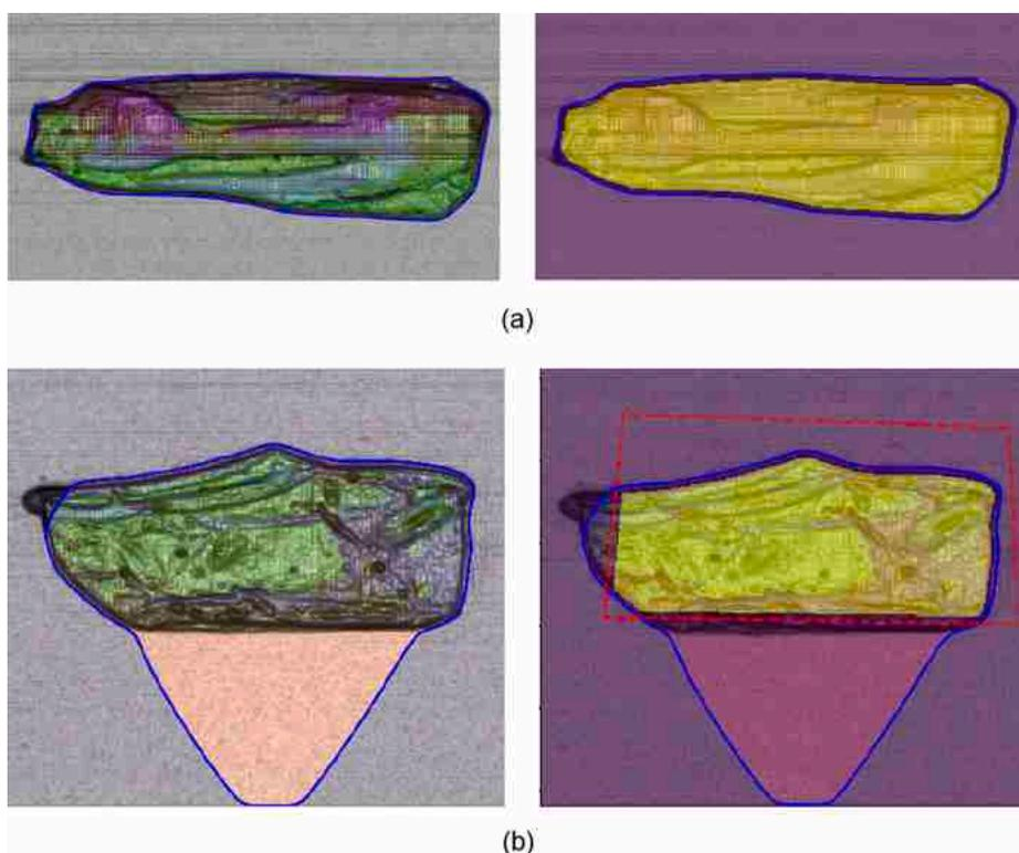
**Fig. 2.** Spectra extraction with self-developed semi-automated process. (a) Data extraction without manual selection; left: automatic object detection result; right: extracted area after erosion (in yellow). (b) Data extraction with manual selection; left: automatic object detection result; right: extracted area (in yellow), blue line is the automatic detected contour and red line is manual selection.
