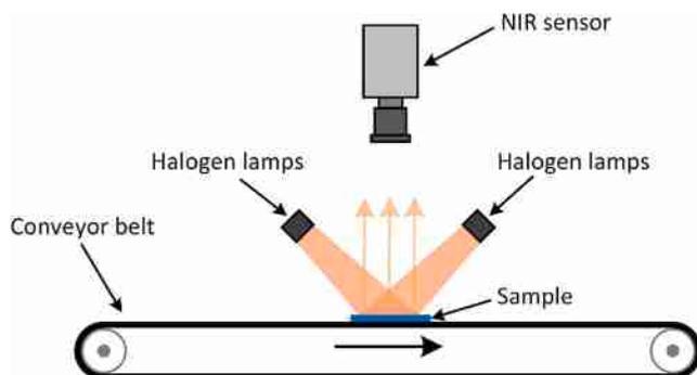
Fig. 1. NIR sensor and illumination setup.
